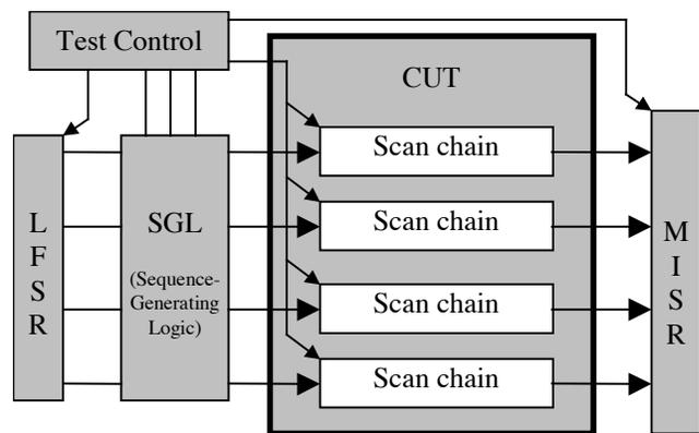
**Figure 2:** Target structure of deterministic BIST scheme
