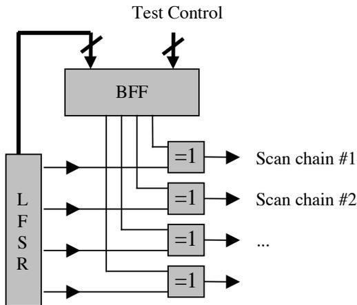
Figure 3: Sequence-Generating Logic
