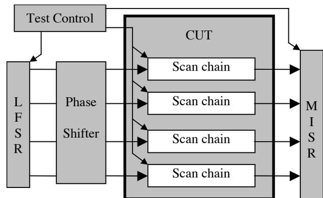
Figure 1: STUMPS architecture with phase shifting logic
