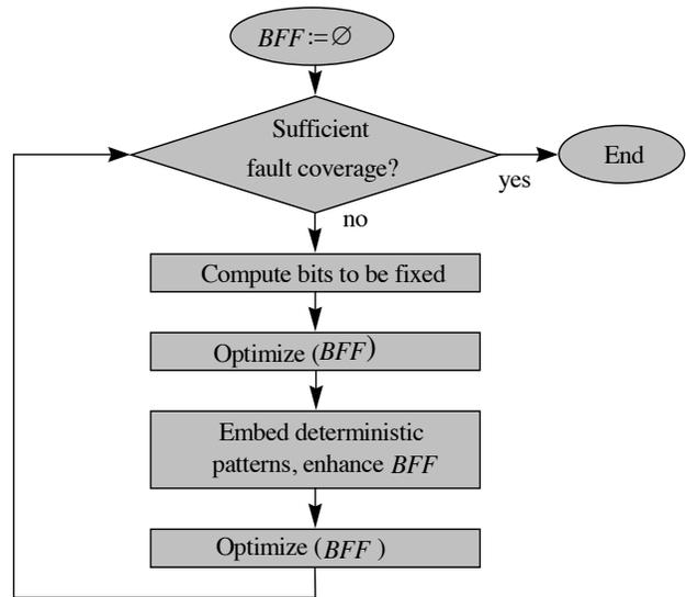
Figure 4: BFF synthesis algorithm
