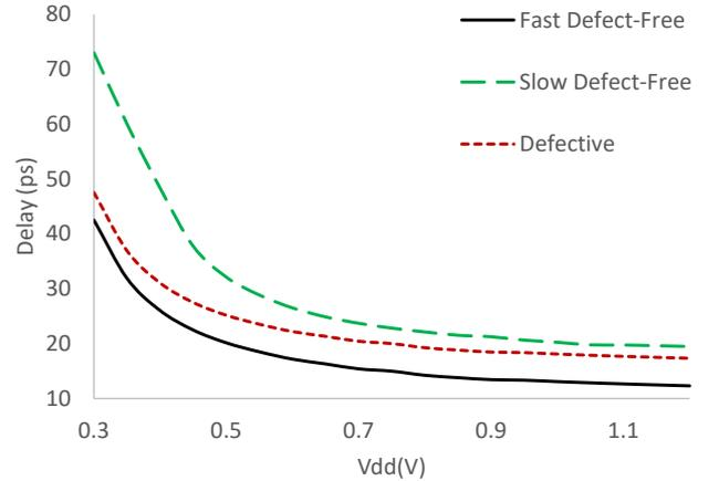
Fig. 3. Timing behavior of two corner instances of a NAND gate vs. a defective cell
