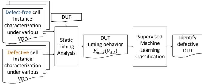
Fig. 1. Overall flow of defect identification based on STA
