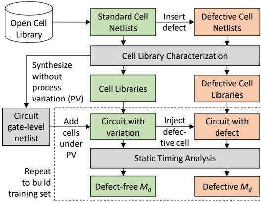
Fig. 4. Overview of our training data generation flow using standard cell characterization and STA.
