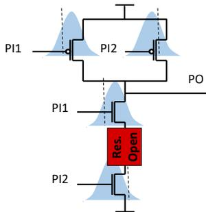
Fig. 2. NAND cell with a resistive open injected
